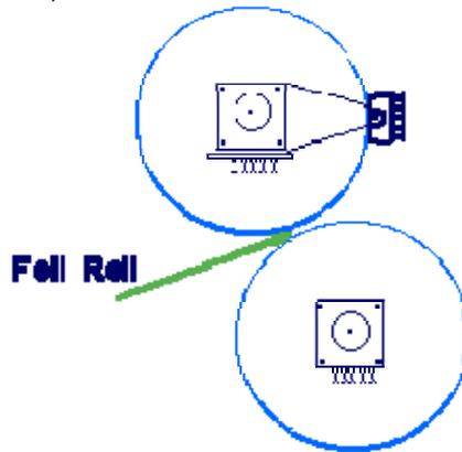
4. Make sure the cutting platform is fully lowered. This is the only safe way to make this measurement, plus on some mower-conditioners, raising the platform also opens and separates the rolls preventing an accurate measure of the minimum roll clearance.
