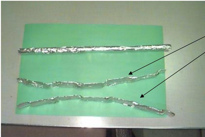
6. The rolls will crush the foil rolls and the minimum roll clearance can be determined by using a digital or dial caliper to measure the thickness of the foil roll. A low-cost digital caliper (~\$40) can be found at Techni-Tool (Part No. 575GA103, 1-800-832-4866). Take several measurements of the thickness along the length of each foil roll and determine an overall average. The measurement should be taken where the “crimp” or smallest clearance occurs as noted in the above figure.
