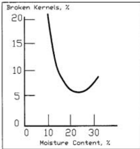
**Figure 8-1. Broken Kernels vs. Corn Moisture Content**
