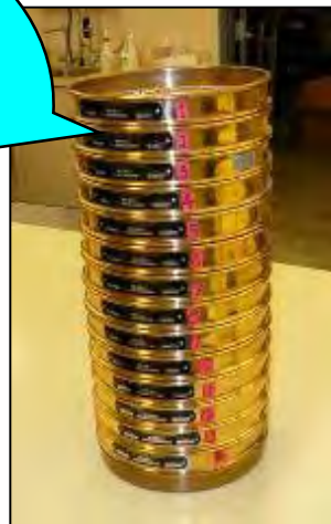
3 – Put the material on the remaining sieves thru the normal K-State grain sieves to better quantify the kernel particle size without interference from non-grain material (cob, husk)
